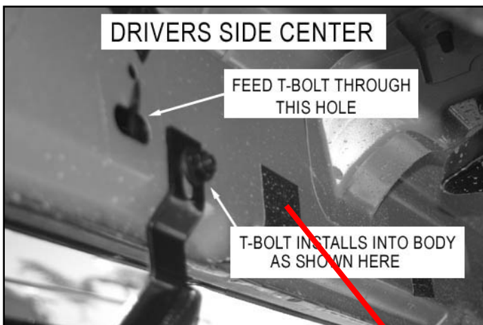
Figure 1.3 –Driver-Side Front Assembly View (1500/2500/3500 Series set-up shown) Attach center support bracket as shown in Fig.3-4. Place hooked T-bolt through body with threaded stud through hole. Secure bracket to bolt using 3/8 nut, lock-washer, and flat washer. Attach side bar to center support bracket with 3/8 bolt, lock washer, and flat washer
