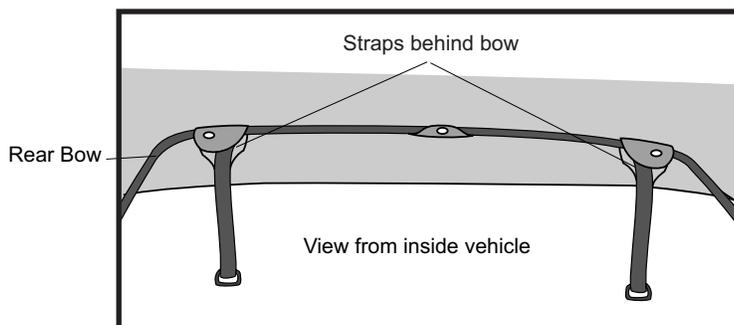
Make sure that the straps sewn into the rear of the top are behind the rear bow.
