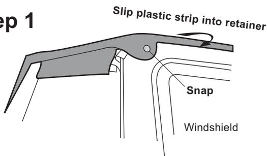
Lay the main skin out on the vehicle and insert the plastic strip into the channel over the front windshield. Now snap the front two snaps. Open the hook and loop flap on the sides over the front doors
