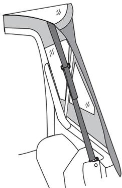
Install the tension strap through the loop on the strap sewn into the top. Pull tight and secure with hook and loop.
