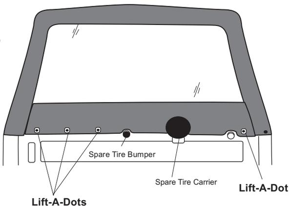
Snap the snaps on the bottom of the side panels from front to back.
