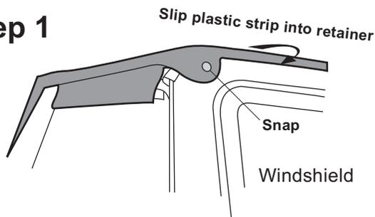
Lay the top out on the vehicle and insert the plastic strip into the channel over the front windshield. Now snap the front two snaps. Open the hook and loop flap on the sides over the front doors
