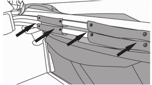
7) Open the top assembly into its up position and latch the top back on the header. Inside the top the velcro bow wrap should be positioned to install on the middle bow by wrapping it around and fastening the velcro.
