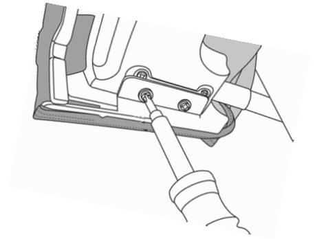
6) Drape the top material over the bow assembly while it is in the up position to initially position the fabric in the approximate location it will be installed. Then fold the bow assembly and top down onto the rear of the vehicle. Position the fabric so the flaps that get screwed to the mid and rear bow are in their correct positions. Install the 8 screws as shown.
